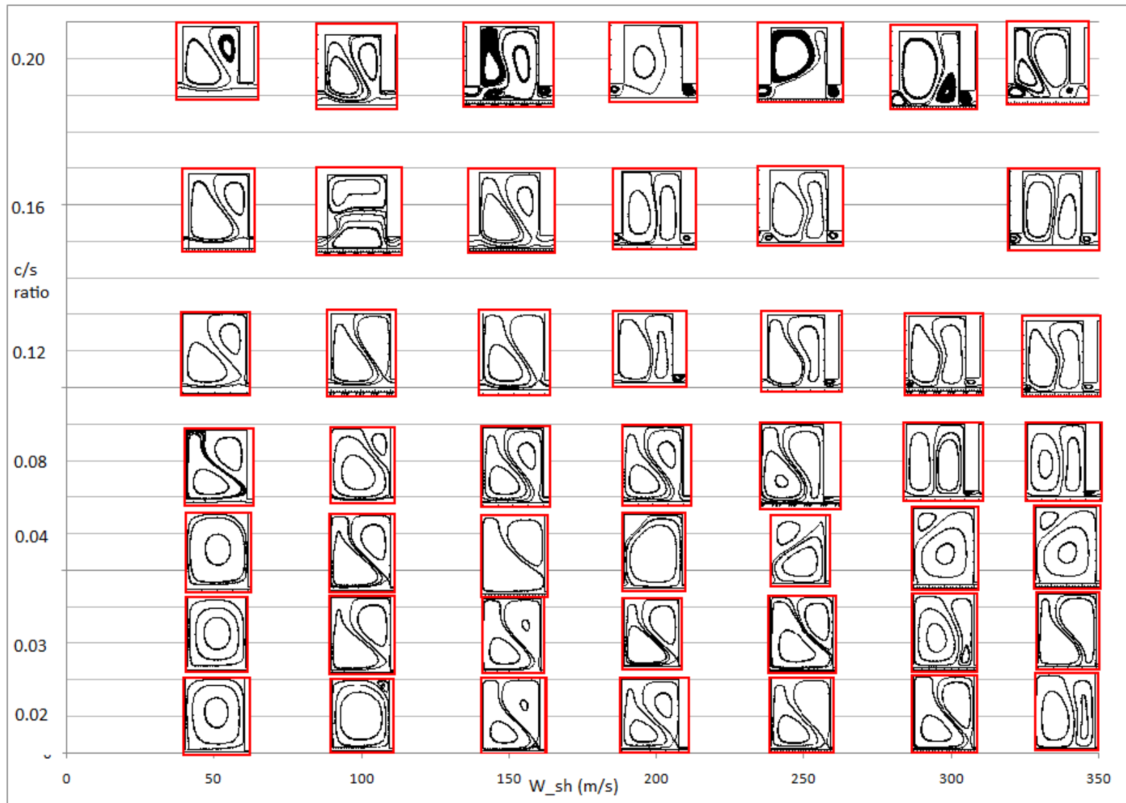
Figure 9. Different streamlines with varying clearance for tooth on stator.
