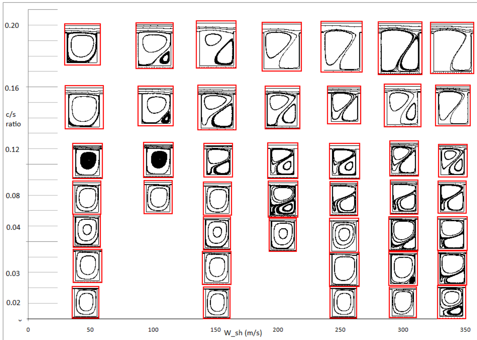
Figure 39. Streamlines with varying c/s ratio for tooth on rotor seal; compressible flow; c = 0.10 mm, w = 1 mm, h = 5 mm, s = 5 mm.
