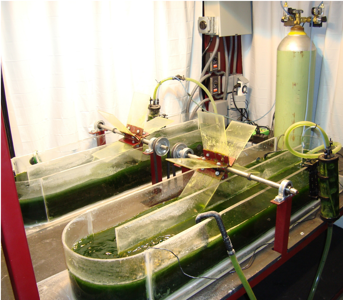
Figure 3: Micro-raceway algae ponds used for light and temperature effects studies.
