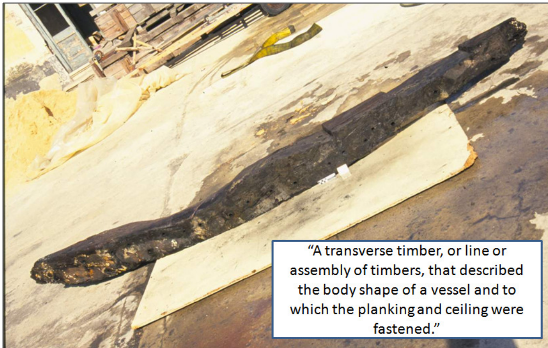
Figure 7.5. Photograph of a frame along with its definition. Photograph courtesy of CMAC.
