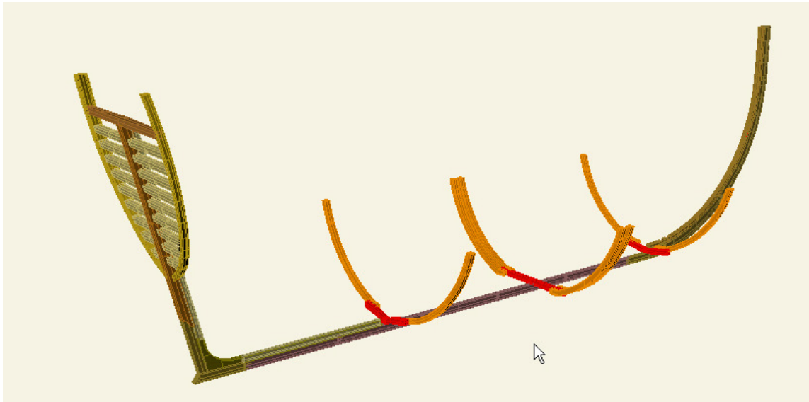
Figure 5.25. Construction sequence (master frame and almogama). Courtesy Alex Hazlett, CMAC.
