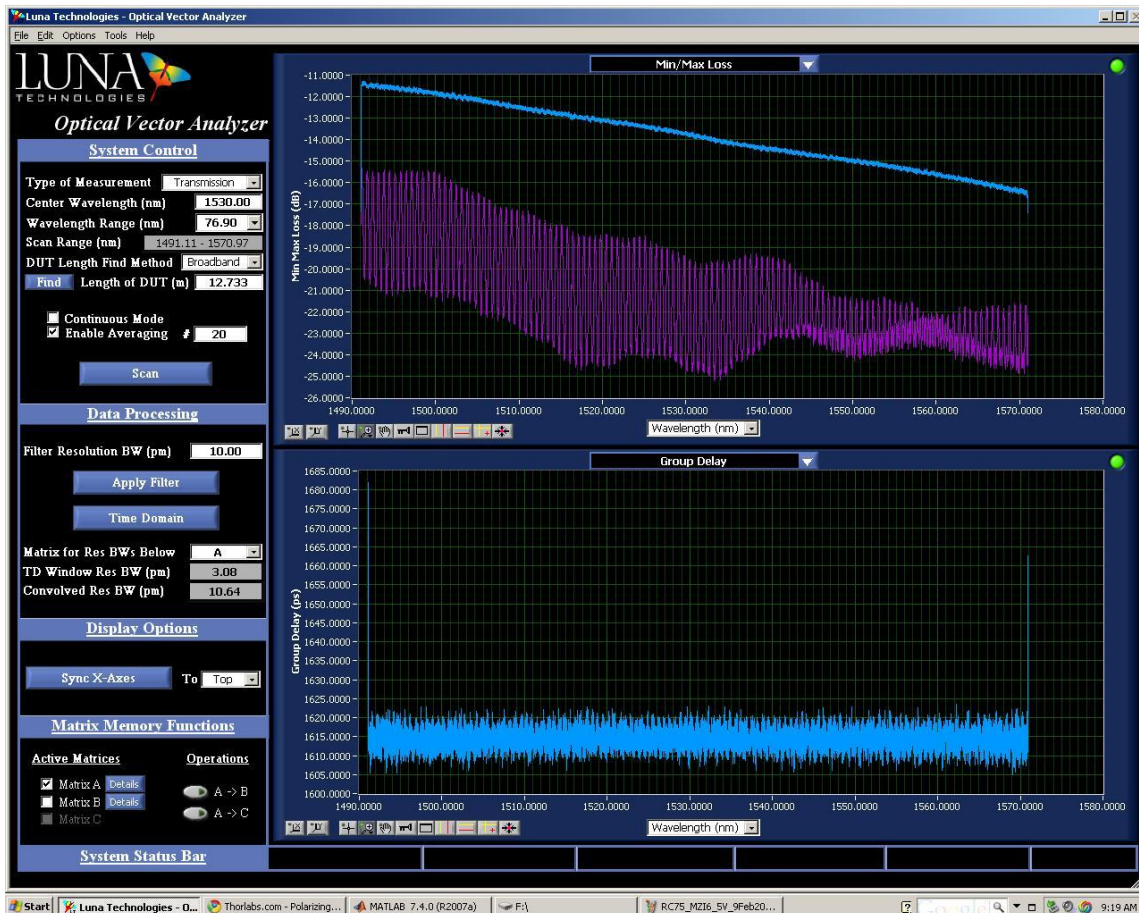
Fig. 34 A sample optical vector analyzer measurement.
