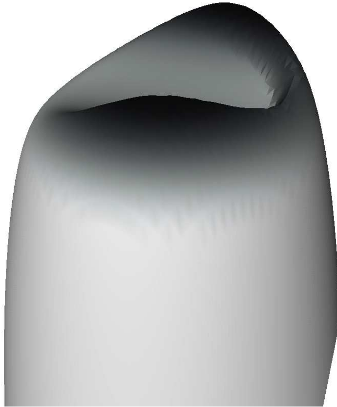
Figure 4.4: Example film thickness solution across an EHL point contact. Minimum non-dimensionalised film thickness: 0.14
