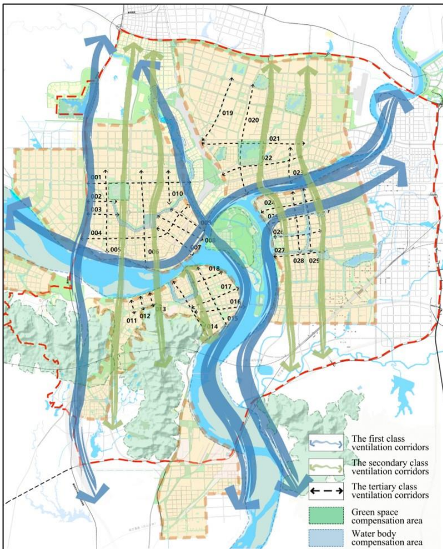
Figure 9. Urban ventilation corridor planning in Xiangyang
