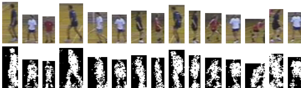
Figure 4.9: A sample from the set of positive examples of bounding boxes well-centred on a player and corresponding foreground/background images.
