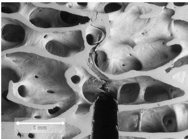
Fig. 1. Crack growth emanating from the man-made notch as in the SENB FT tests of Cook and Zioupos (2009) and Ding and Hvid (2000). Following application of bending moments on either side the notch opens up and the trabeculae ahead of it start snapping. The deformation and crack growth was stopped as soon as this first critical load was reached. The load was used to define the K_{\text{C}} value (initial notch width \sim 300 \mu\text{m} ).
