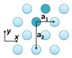
FIG. 2. (Color online) The geometry of the simulated array. NMAG simulations were performed for the two nanowires (shaded dark) as part of a quasi-infinite array created by tessellating virtual copies of the two nanowires with the primitive lattice vectors  $\mathbf{a}_1$  and  $\mathbf{a}_2$ . The dimensions of the full array were  $\sim 8 \times 8 \times 0.8 \ \mu m$ .
