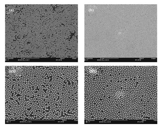
FIG. 1. SEM images of experimentally measured nanowire arrays (a) and (b) with 10 000 magnification; (a1) the same array as (a) with 20 000 magnification; (b1) the same array as (b) with 30 000 magnification.
