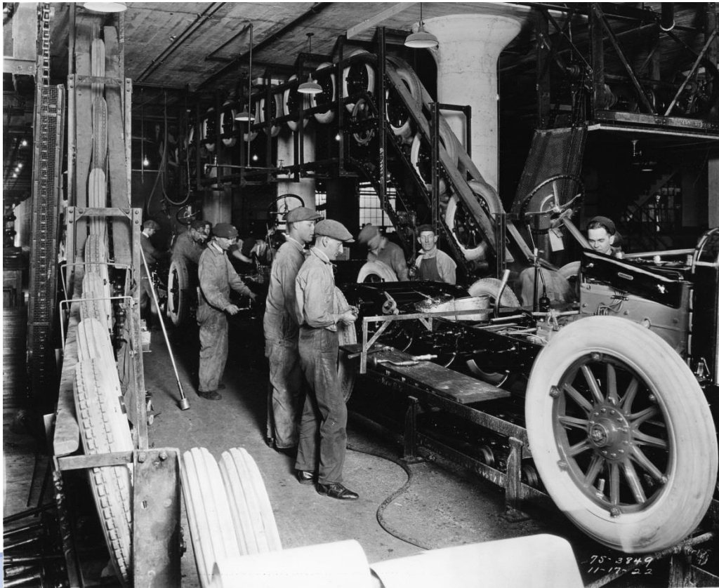
Figure 1. A view from GM automobile factory which shows assembly line workers attach tires to GM vehicles
