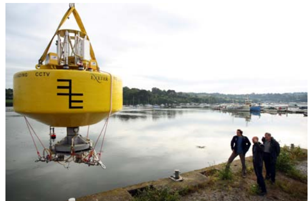
Figure 1 Launch of Mooring test buoy
