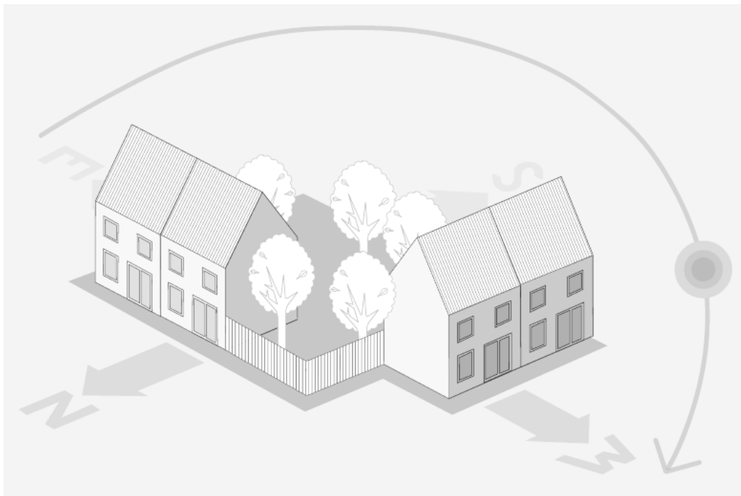
Figure 4-2: An example sun path, and consequent solar heat gains at the building surfaces, illustrating the need to factor building orientation into designs
