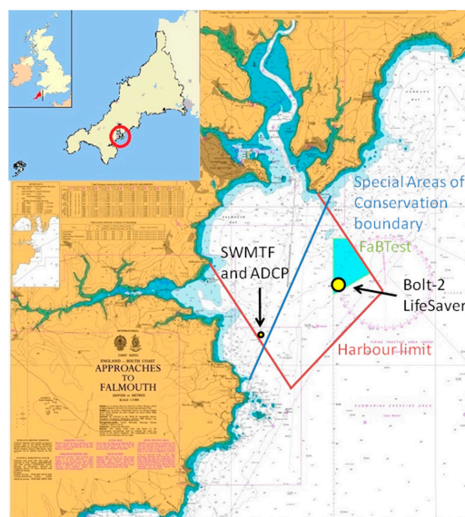
Figure 1. South West Mooring Test Facility (SWMTF) and the Falmouth Bay Test Site (FaBTest) locations, adapted from the United Kingdom Hydrographic Office (UKHO) admiralty chart. ADCP: acoustic Doppler current profiler.
