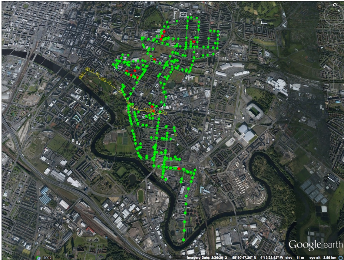
Figure 57 - Testing Dalmarnock Model, Green features are combined, Red are wastewater, and Yellow are storm flow.
