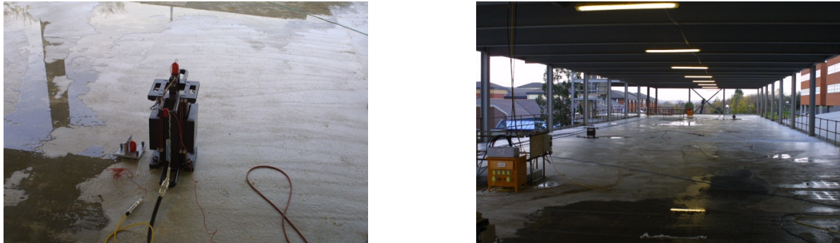
Fig. 5: The left photo shows a shaker and accelerometer that was used in phase 1 and the right plot shows the bare structure of phase 1
