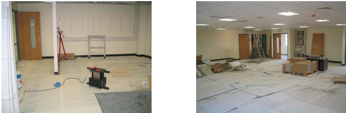
Fig. 6: The left photo shows a shaker used in Phase 3 and the right photo shows one of the largest partitioned out rooms from Phase 3
