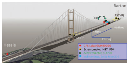
Figure 1. Humber Bridge instrumentation.
