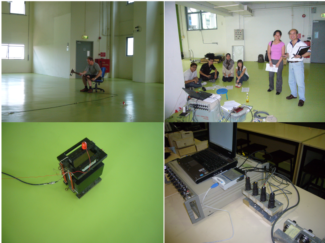
Figure 3: Modal testing. Clockwise from top left: Hammer test using instrumented hammer and IEPE sensors; helpers and observers in 2000-3L-4; Quartz-flex accelerometers, signal conditioner and National Instruments compact DAQ; APS400 shaker.
