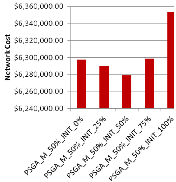
Figure 6. Pipe Smoothing Initialisation Rate Results for PSGA M 50% on Hanoi, Mean Best Feasible Solution Cost
