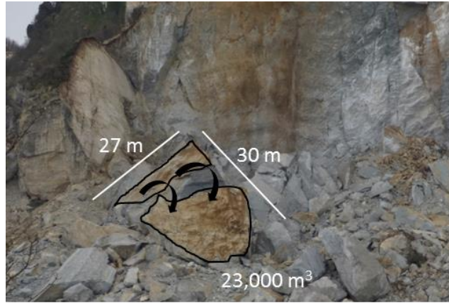
Fig. 9 Blocks in the deposit area, which appear to have been broken on impact with the ground
