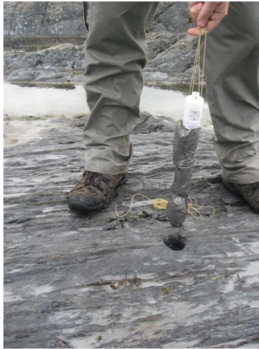
Figure 4.2: Images of the weighted RBR TWR-2050P pressure transducer about to be inserted into the deployment hole at the central inner shore platform.
