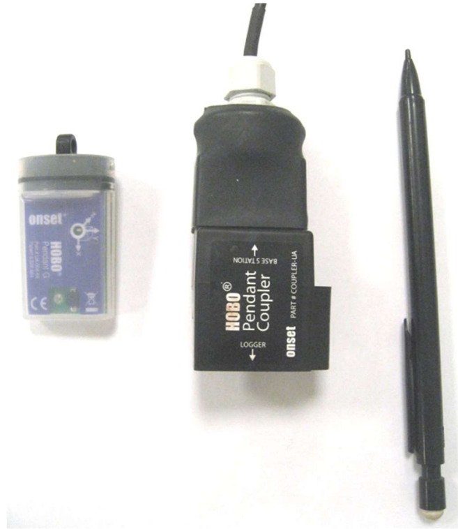
Figure 3.5: Image of (left) Onset Pendant G Data Loggers (UA-004-64) and (centre) BASE U-1 optical USB and coupler device.
