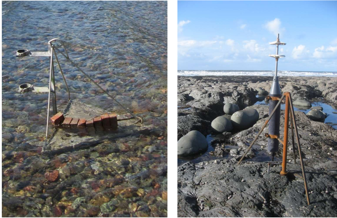
Figure 3.6: Images of the MAVS and its mooring frames at Flathead Lake and Abbotsham. Left: MAVS mooring frame used in the Flathead Lake experiments (without MAVS device and not positioned correctly). Right: Custom designed mooring frame holding the MAVS device on the shore platform at Abbotsham.
