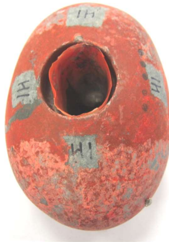
Figure 3.4: Image of an adapted ML clast (A01) from Abbotsham, displaying the motion logger mould. Scale: Cored hole is 35 mm in diameter.
