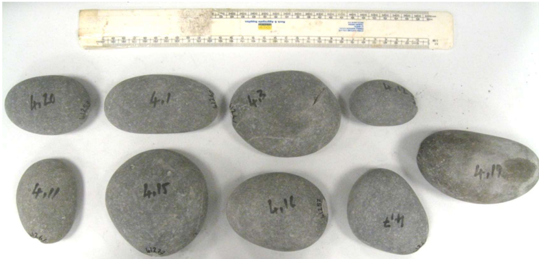
Figure 4.4: photo of a selection of clasts displaying the marine epoxy cap after being fitted with RFID tags. Scale: The ruler is approximately 270 mm in length.
