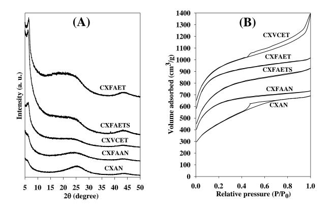
Figure 2. Powder XRD patterns (A) and nitrogen sorption isotherms (B) of microporous carbon templated from zeolite 13X under various conditions by combination of liquid impregnation with furfuryl alcohol and CVD with ethylene. For clarity, the isotherms for sample CXFAET and CXVCET were offset by 50 and 200 along the y axis, respectively.
