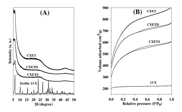
Figure 1. Powder XRD patterns (A) and nitrogen sorption isotherms (B) of microporous carbon templated from zeolite 13X under various conditions via CVD with ethylene as carbon precursor.
