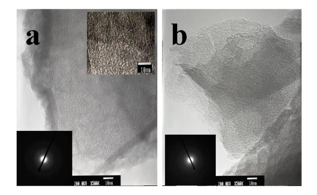
Figure 5. Representative TEM images of microporous carbon materials templated from zeolite 13X. (a) CXET and (b) CXFAET.
