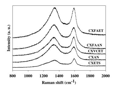
Figure 3. Raman shifts of microporous carbon materials templated from zeolite 13X under various synthesis conditions.
