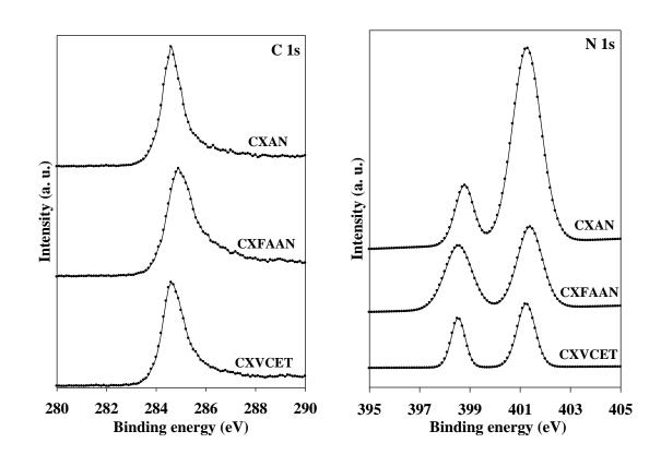
Figure 6. XPS of C1s and N 1s of microporous carbon materials templated from zeolite 13X under various preparation conditions.
