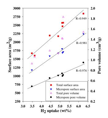
Figure 8. Hydrogen uptake capacities of zeolite 13 templated carbon materials as a function of total surface area, micropore surface area, total pore volume and micropore volume.
