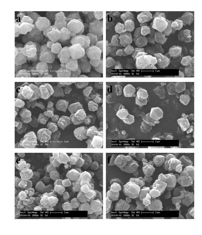
Figure 4. Representative SEM images of microporous carbon materials (b-f) templated from zeolite 13X (a) under various synthesis conditions; (b) CXETD, (c) CXET, (d) CXFAET, (e) CXFAAN and (f) CXVCET.
