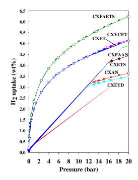
Figure 7.  $H_2$  uptakes of microporous carbon templated from zeolite 13X under various preparation conditions.
