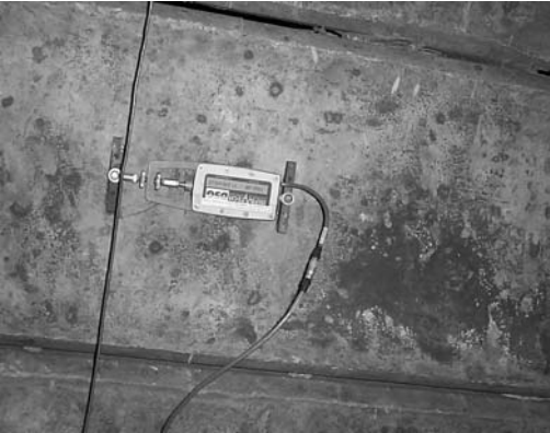
(b) Demountable strain gauge
