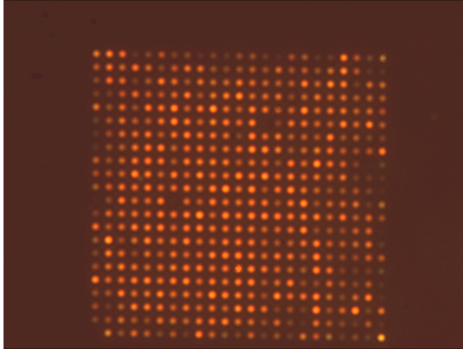
Figure 2.8: Colour image taken using a CCD coupled to an optical microscope illustrating the resonantly scattered light from silver nanoparticles. The scattered light can be observed using an optical microscope as the scattering cross-section of each disc is larger than its geometric cross-section. Particles are arranged in a 50\ \mu\text{m} \times 50\ \mu\text{m} square array with a 2\ \mu\text{m} pitch to avoid particle interactions.
