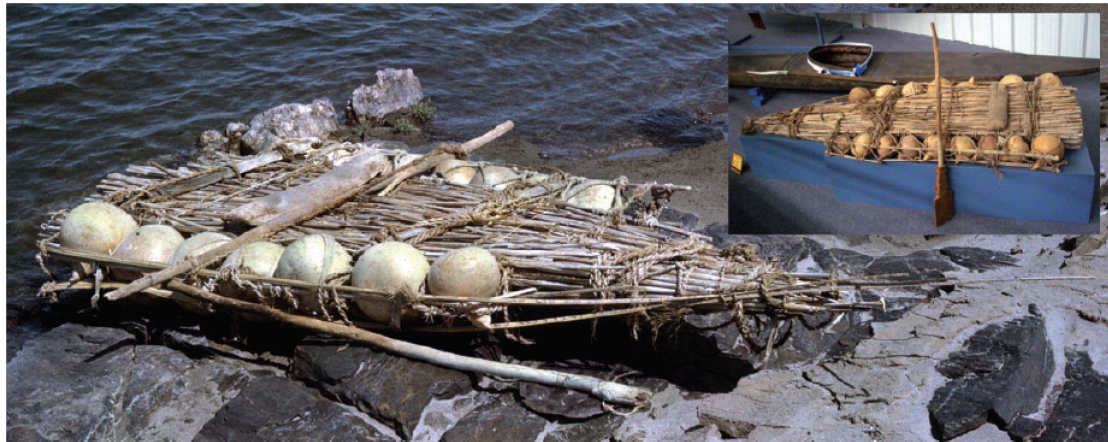
Figure 11. A geyyi raft at Semna, Sudanese Nubia, comprising bundled reeds with bottle gourds to provide lateral stability (Image courtesy of Herman Bell, University of Exeter). The inset shows the example at the Mariners' Museum, Newport News, Virginia, USA (Image courtesy of the Mariners' Museum).
