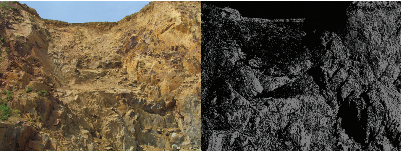
Figure 9. Split FX software point cloud image of the upper region of the western face from the 2011 scanning survey (right), and a photograph of the same slope (left). Figure 10 shows the stereoplot derived from the laser scanning of this face.
