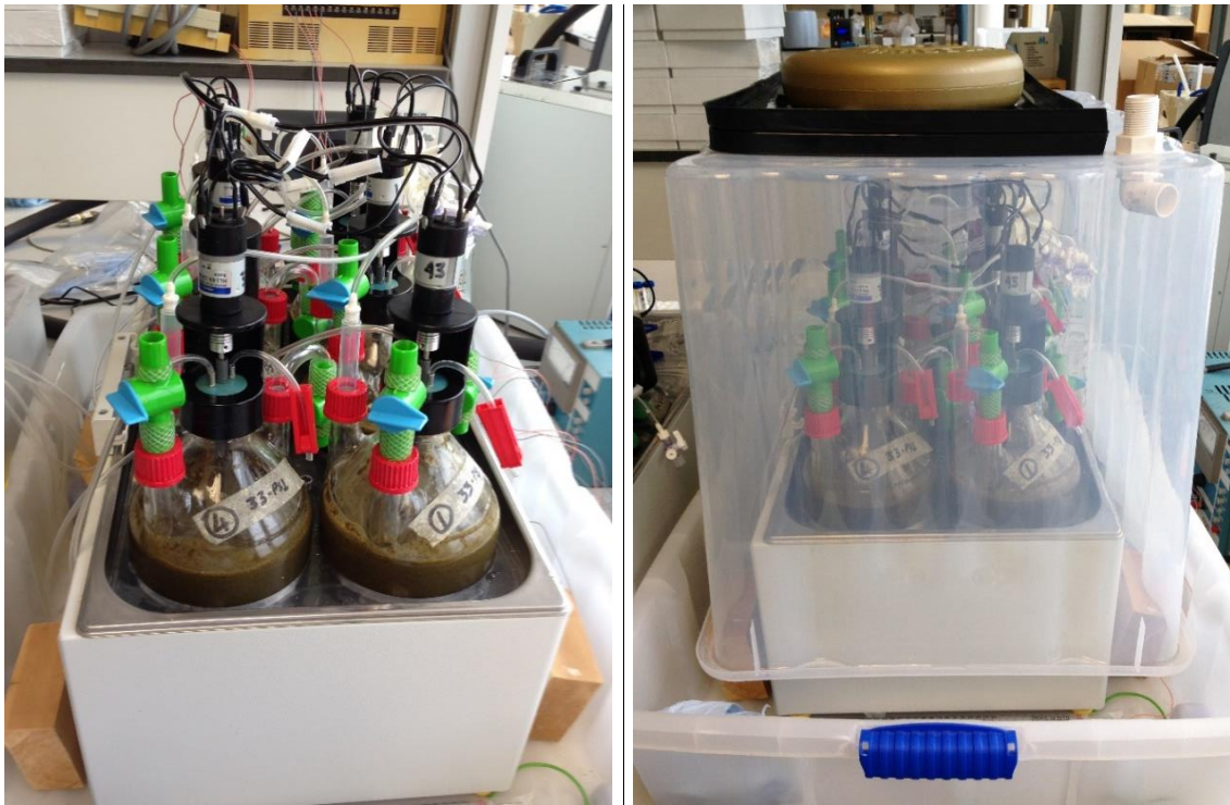
Figure 49 – Adapted Duran flask and AMPTS II with safety features installed
