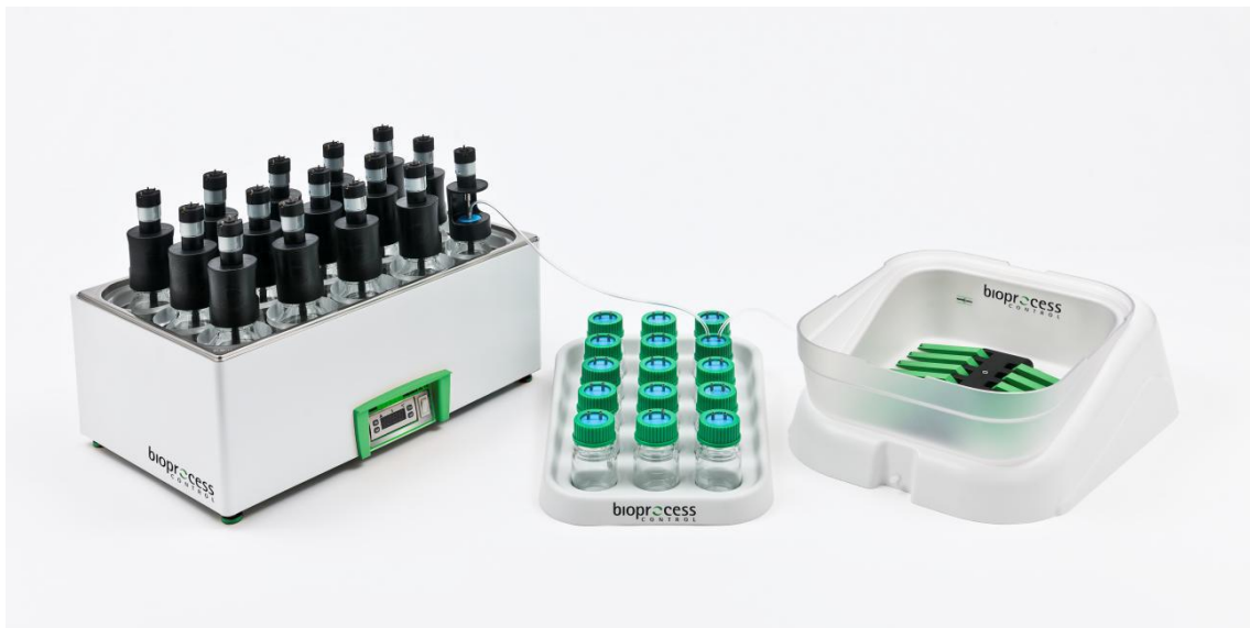
Figure 30 – Automatic Methane Potential Test System II (courtesy of Bioprocess Control Sweden AB)
