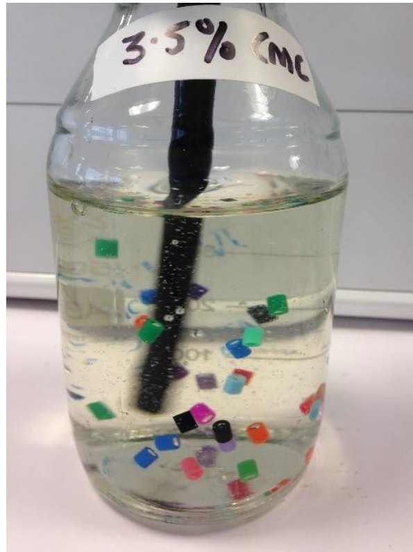
Figure 3 – Visual assessment of regional mixing across a digester using suspended coloured beads
