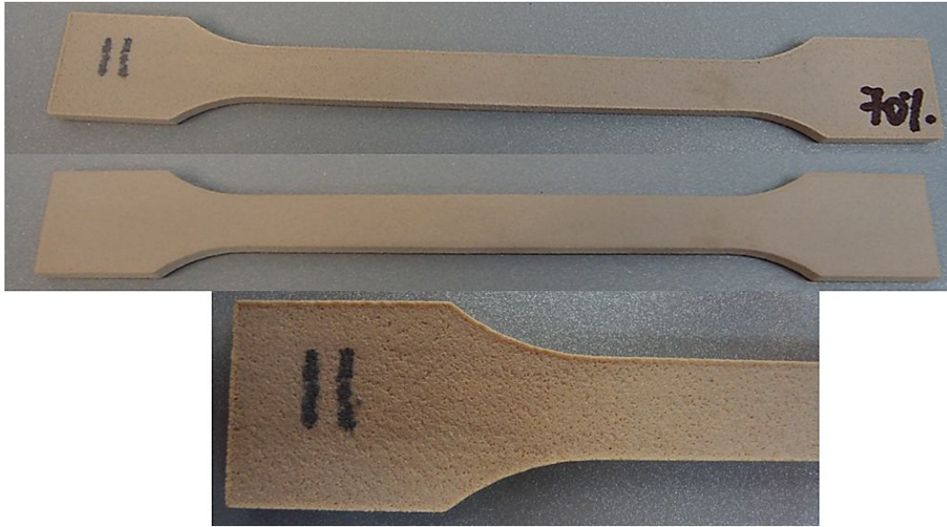
Figure 97. Build for testable HT laser sintered PEEK samples: sample G, manufactured at 70% laser power in respect to the standard EOS laser exposure settings
