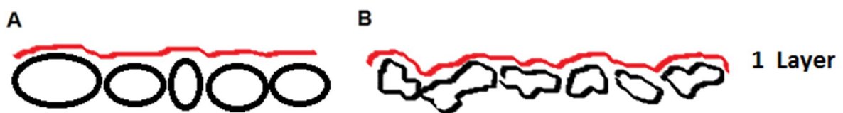
Figure 164. Surface roughness of the one layer samples and particle morphology in the powder bed
