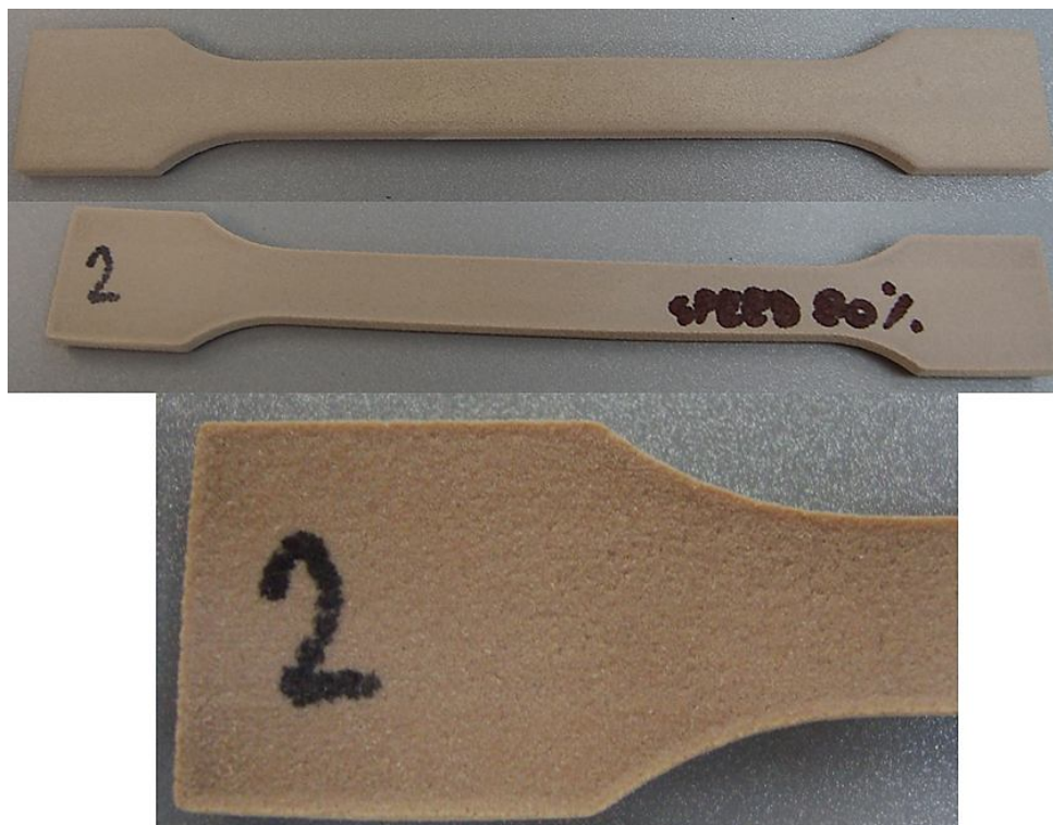
Figure 103. Build for testable HT laser sintered PEEK samples: sample M, manufactured at 80% scan speed in respect to the standard EOS laser exposure settings
