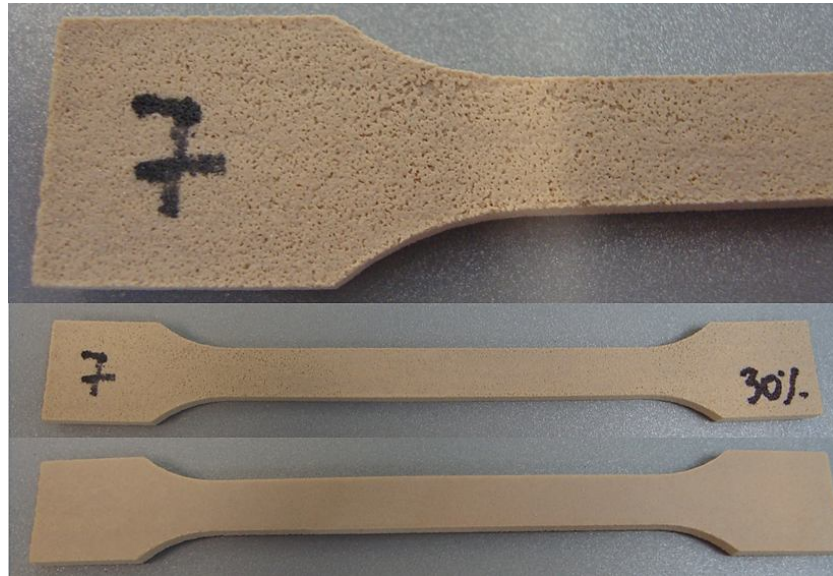
Figure 93. Build for testable HT laser sintered PEEK samples: sample C, manufactured at 30% laser power in respect to the standard EOS laser exposure settings
