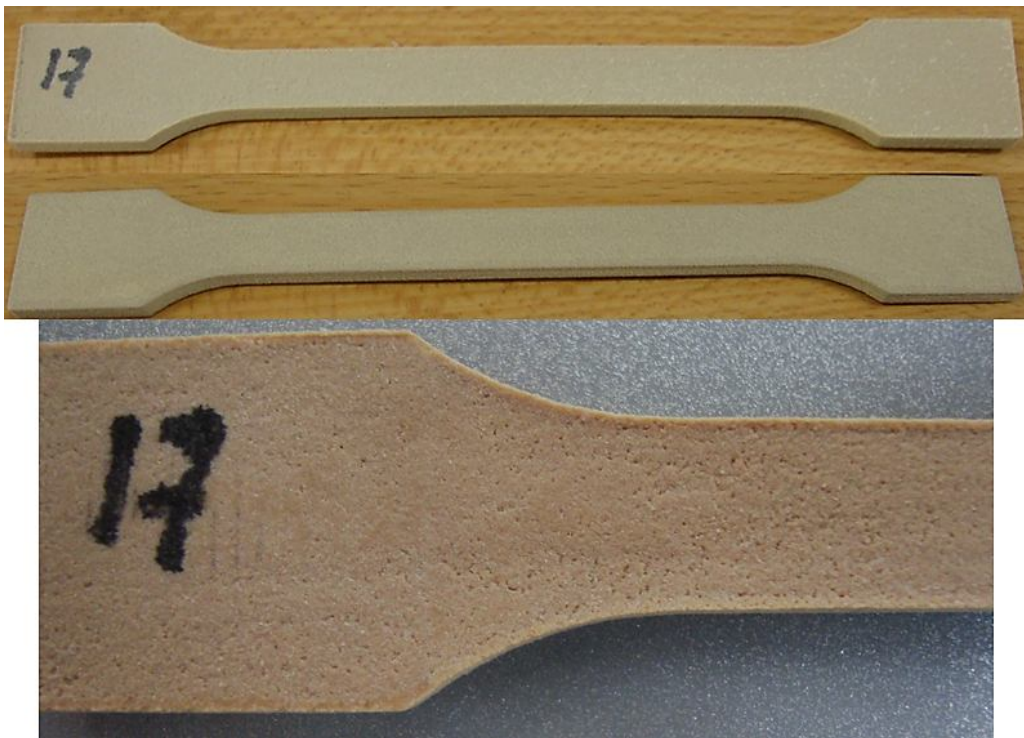
Figure 98. Build for testable HT laser sintered PEEK samples: sample H, manufactured at 80% laser power in respect to the standard EOS laser exposure settings
