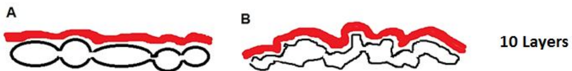
Figure 165. Surface roughness of the ten layer samples and particle morphology in the powder bed
