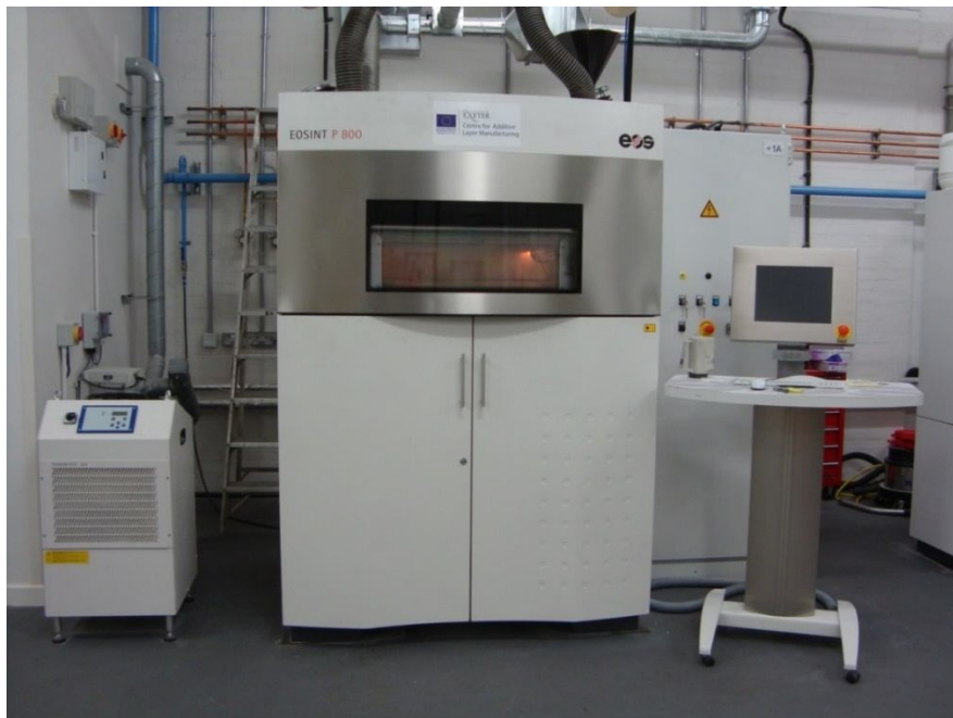
Figure 75. The EOSINT P 800 system
