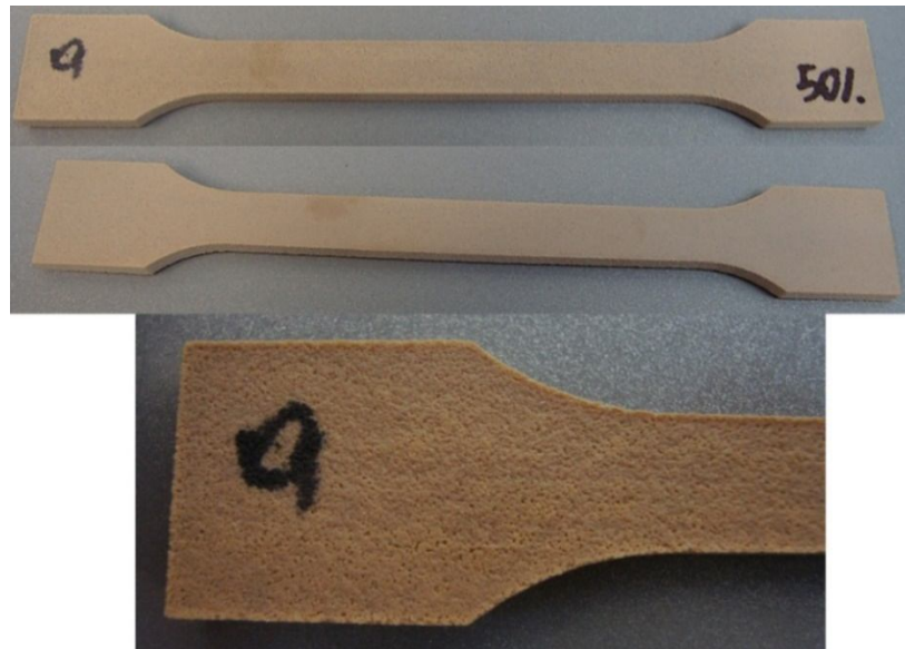
Figure 95. Build for testable HT laser sintered PEEK samples: sample E, manufactured at 50% laser power in respect to the standard EOS laser exposure settings
