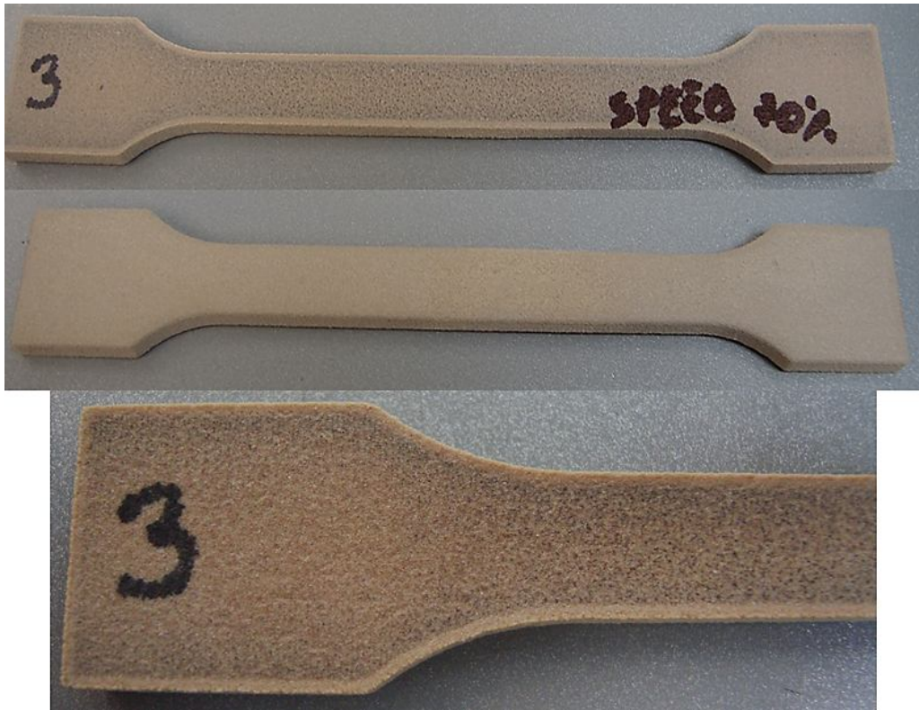
Figure 104. Build for testable HT laser sintered PEEK samples: sample N, manufactured at 70% scan speed in respect to the standard EOS laser exposure settings Sample N
