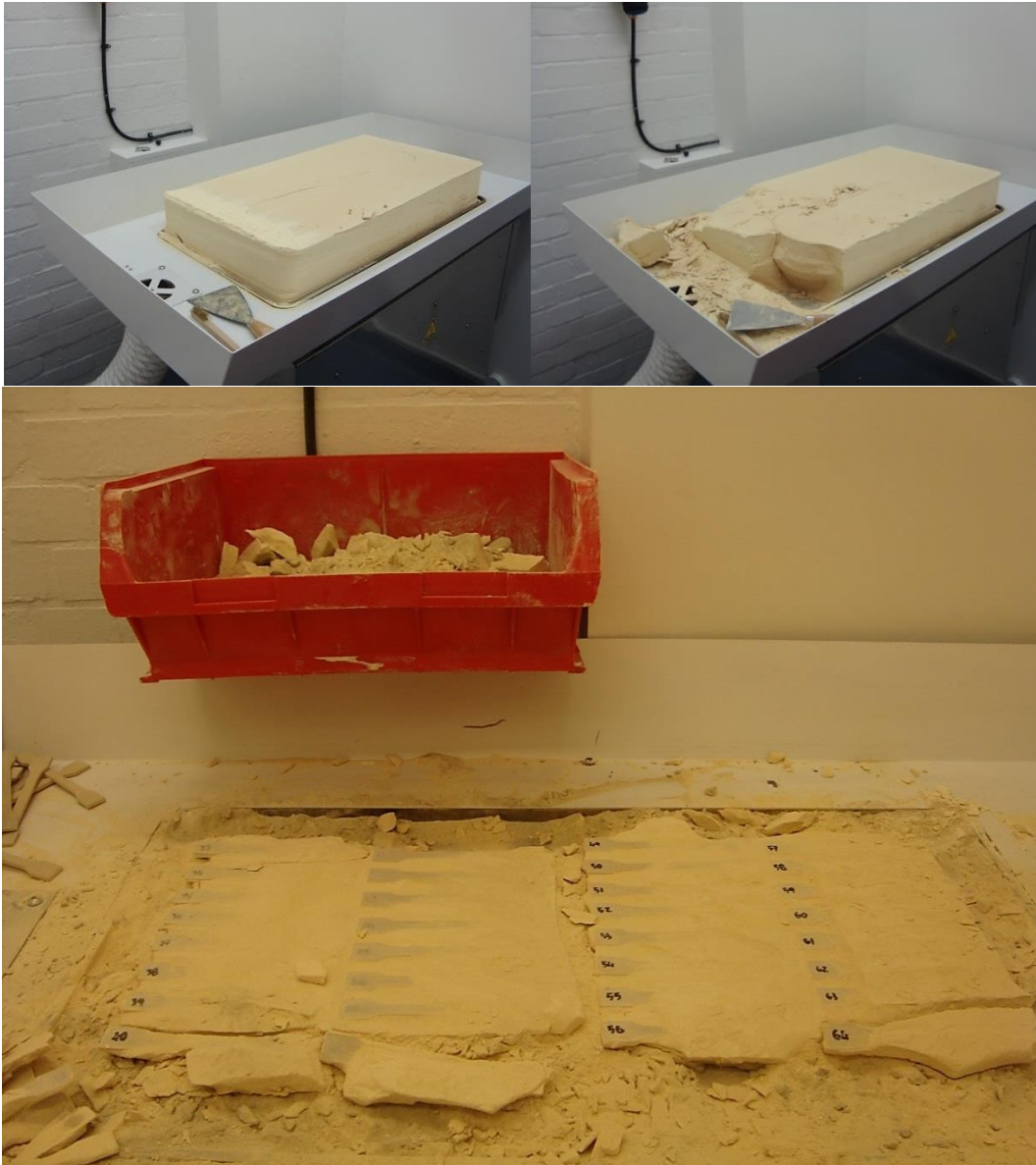
Figure 78. Powder cake and removal of HT laser sintered PEEK parts (tensile testing bars) from the powder bed
