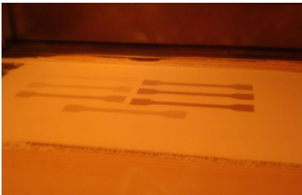
Figure 89. Build for testable samples. Each tensile bar was sintered with individual values of laser exposure corresponding to individual values of ED.
