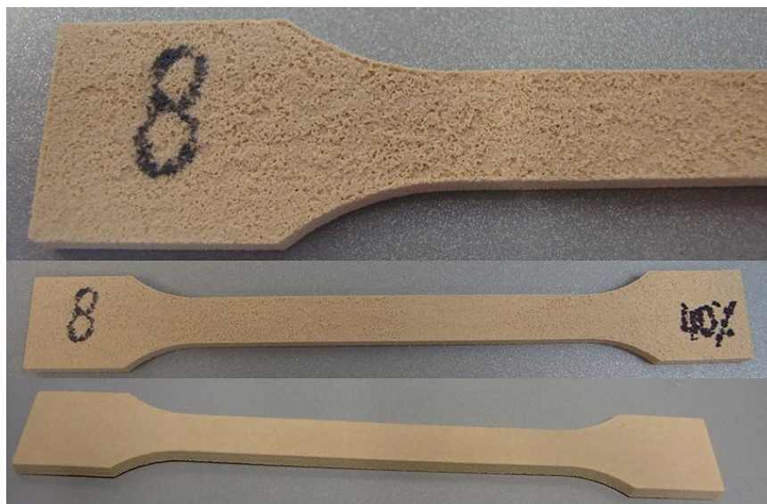
Figure 94. Build for testable HT laser sintered PEEK samples: sample D, manufactured at 40% laser power in respect to the standard EOS laser exposure settings
