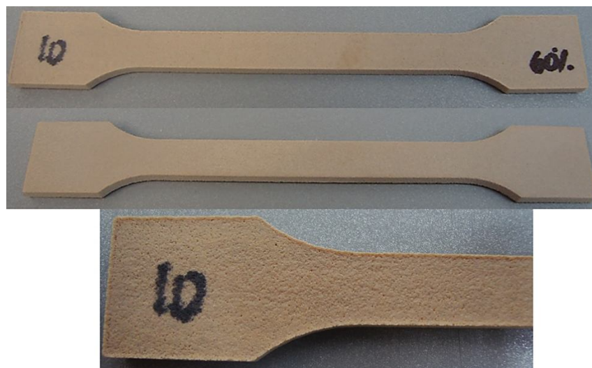
Figure 96. Build for testable HT laser sintered PEEK samples: sample F, manufactured at 60% laser power in respect to the standard EOS laser exposure settings
