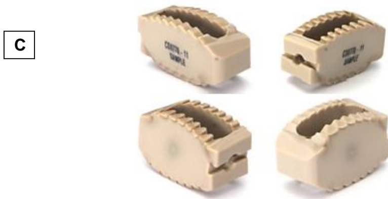
Figure 214. Results of the machines spinal lumbar cages. (A) Numerical results. (B) Load-Displacement profiles (C) Tested specimens
