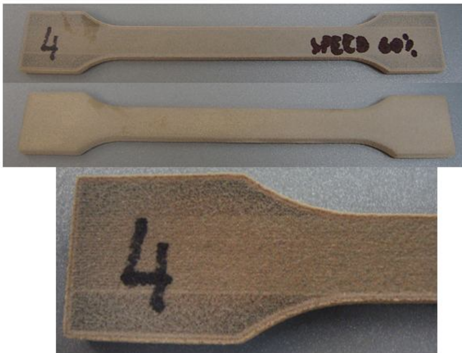
Figure 105. Build for testable HT laser sintered PEEK samples: sample O, manufactured at 60% scan speed in respect to the standard EOS laser exposure settings
