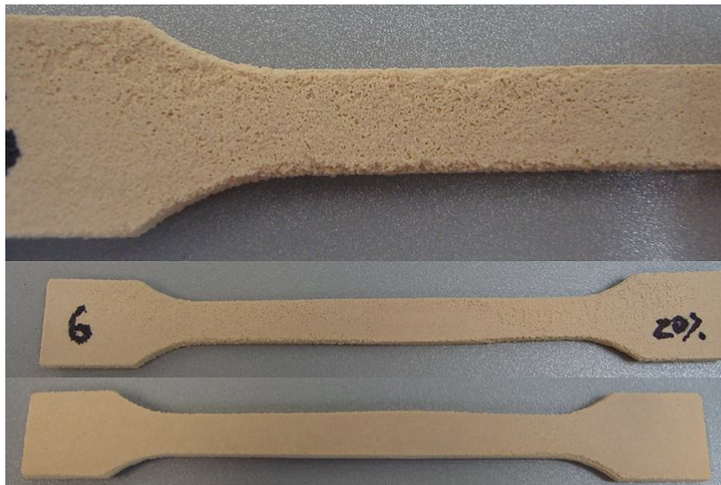
Figure 92. Build for testable HT laser sintered PEEK samples: sample B, manufactured at 20% laser power in respect to the standard EOS laser exposure settings
