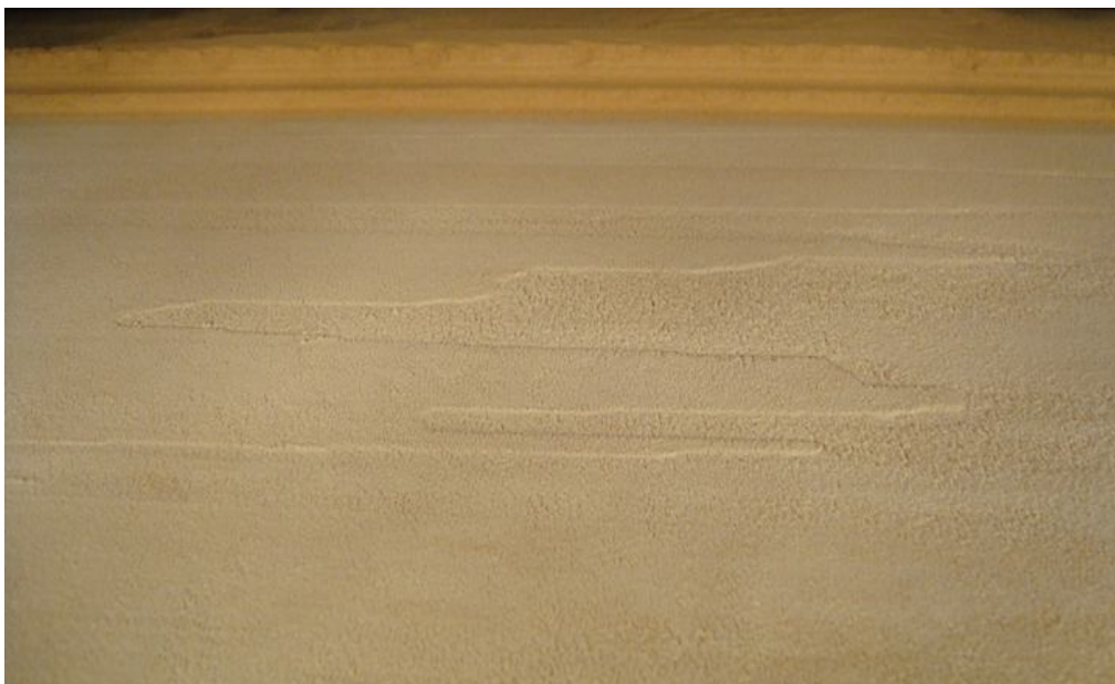
Figure 74. Imperfections in the powder bed of the EOSINT P 800 system. Material: thermally conditioned PEEK 450PF
