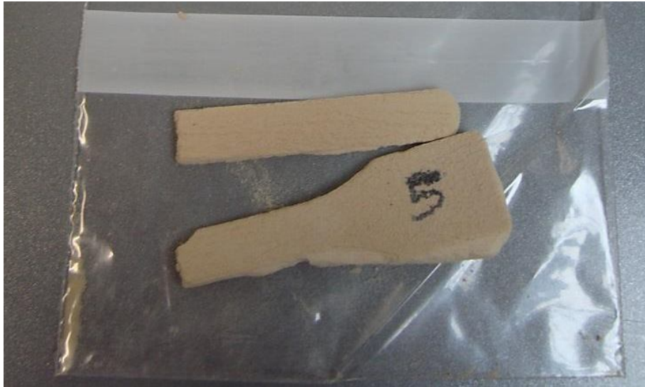
Figure 91. Build for testable HT laser sintered PEEK samples: sample A, manufactured at 10% laser power in respect to the standard EOS laser exposure settings
