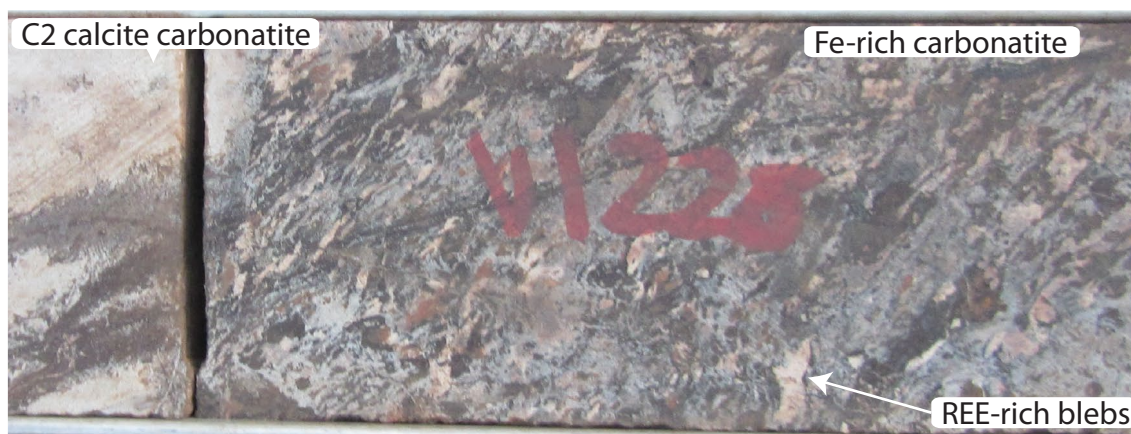
Figure 3.12: Contact between (C3) Fe-rich carbonatite and C2 calcite carbonate in drill core (PX03, 16 m depth). Note the juxtaposition between the banded white and dark carbonatite with the creamy calcite carbonatite (far left).
