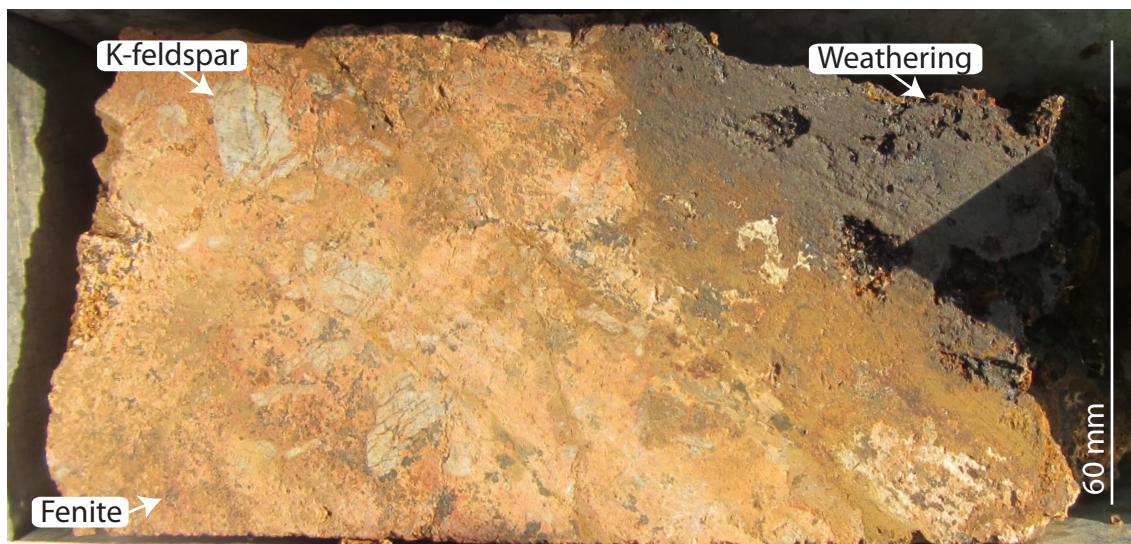
Figure 3.8: Example of fenite from Songwe Hill, with K-feldspar grains. Sample T0185, hole PX003, depth 89.1 m. Thin-section image in Figure 4.4 A, Chapter 4, page 102.
