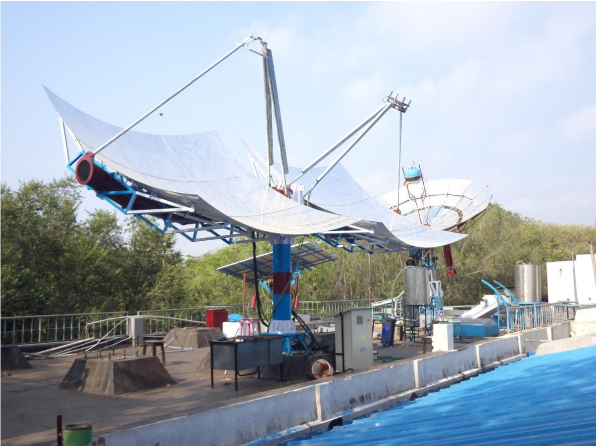
Figure 130 - Experimental setup: the ceramic plate on the left hand side mirror and the receiver on the right hand side one.
