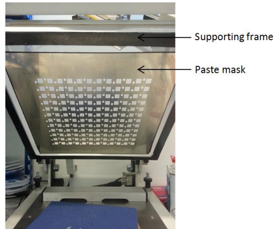
Figure 53 - Image of the paste mask used for the population of the 144-cell assembly.
