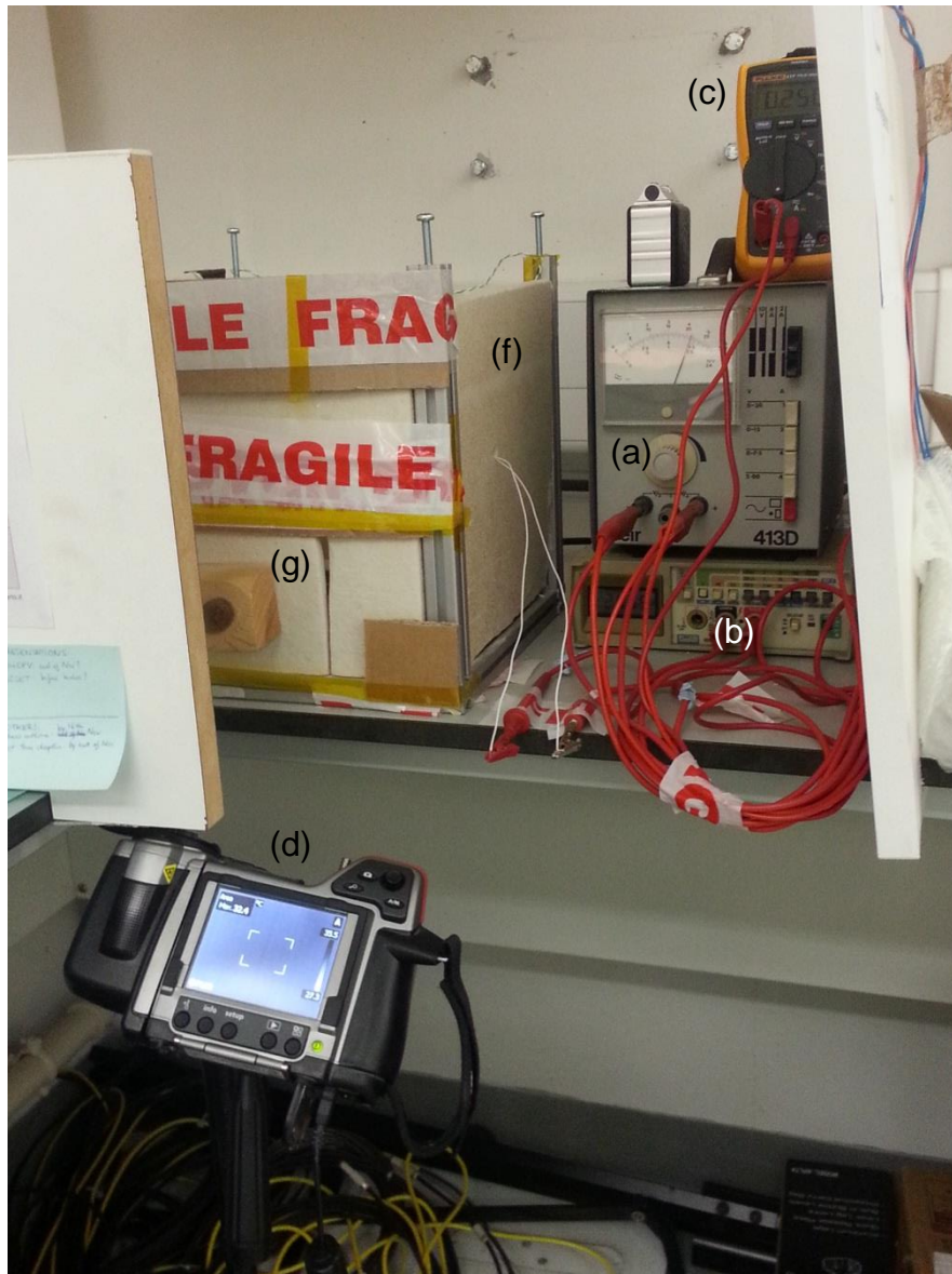
Figure 59 - Picture of the experimental apparatus: (a) the DC power supply, (b) the voltmeter, (c) the ampere-meter, (d) the IR camera, (f) the 25cm×25cm×25cm box, (g) the 10 cm×10 cm removable opening.
