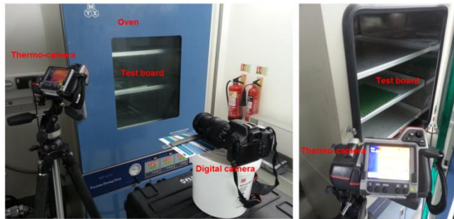
Figure 125 - Setup of the thermal expansion experiment
