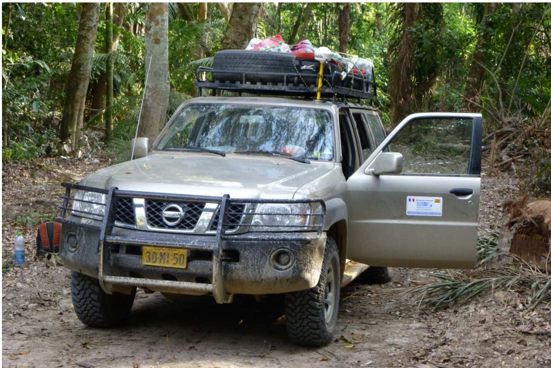
Figure 4.2. Vehicle mounted with differential GPS at front left, used for kinematic and static floodplain elevation surveys.
