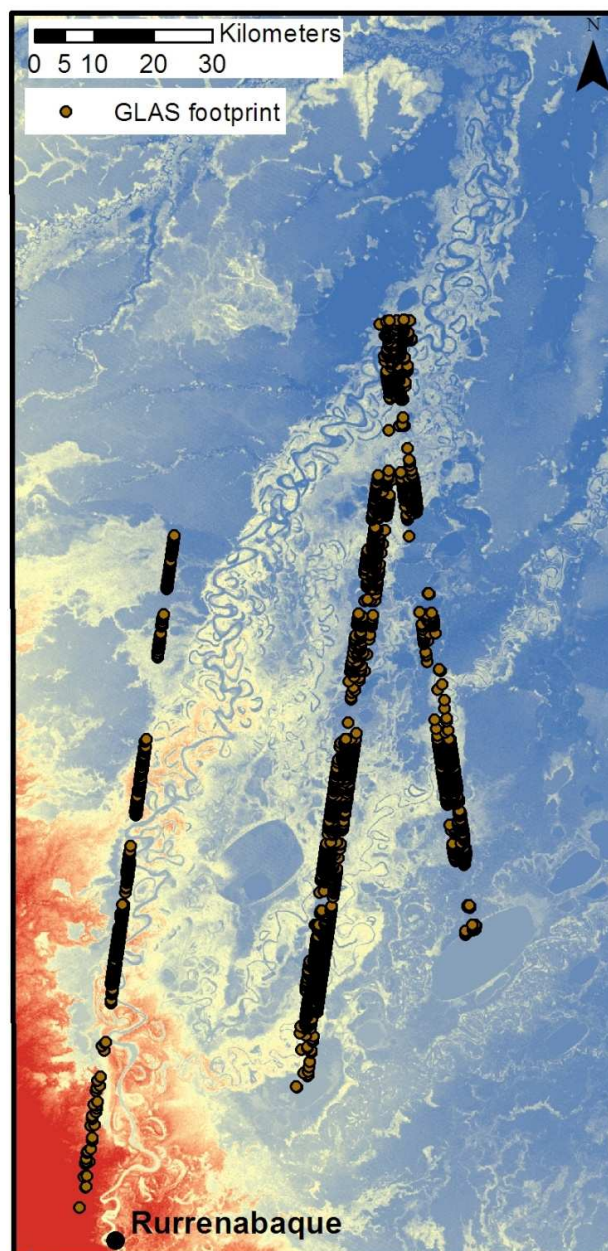
Figure 5.1. Location of GLAS footprints (Saatchi et al., 2011) in the Beni floodplain study area overlain upon the SRTM elevation dataset.
