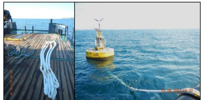
Figure 7: Four tethers for deployment (LH image). Tethers being deployed at SWMFT (RH image).
