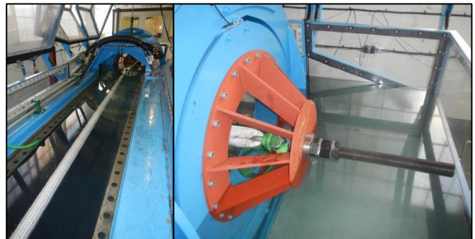
Figure 4: DMaC with a tether fitted and full of water (LH image). The pre-tension adjuster and ‘top hat’ (RH image).
