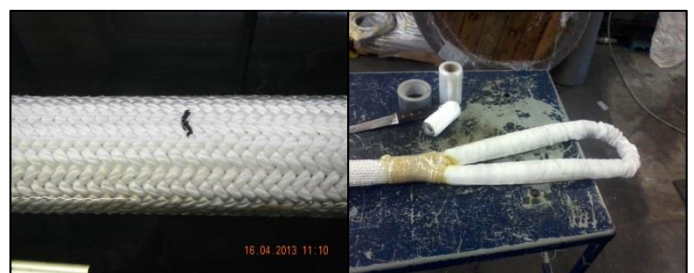
Figure 2: The 48 strand 1x1 braided rope (LH image) and Lankhorst Rope's A3 eye splice (RH image)
