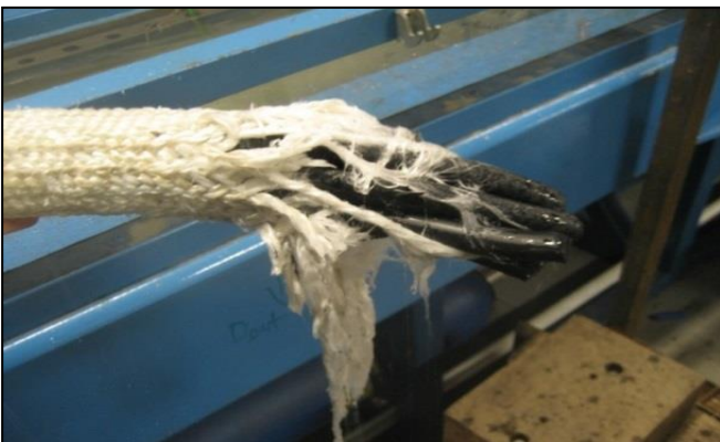
Figure 12: Failed tether under fatigue cycle loading
