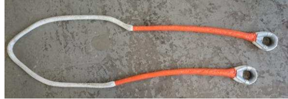
Fig. 6 One of the 30 mm diameter polyamide samples used for DMaC testing
