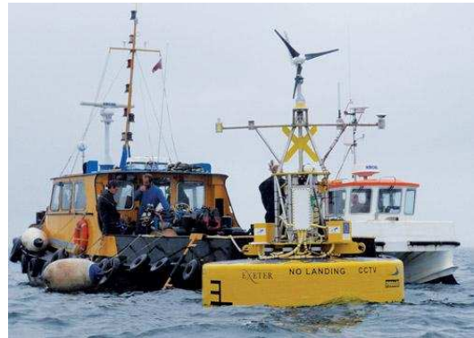
Fig. 7 Deployment of the mooring system at the SWMTF site
