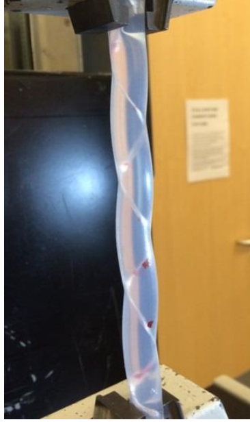
Figure 4: Picture of a typical 3-component auxetic composite in the tensile test.
