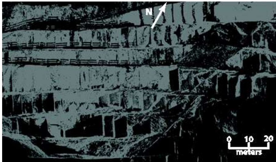
Figure 6. Example screen-shot image of a section of the geo-referenced x, y, z point cloud based on 2012 laser scanning (the scale bar is indicative only)
