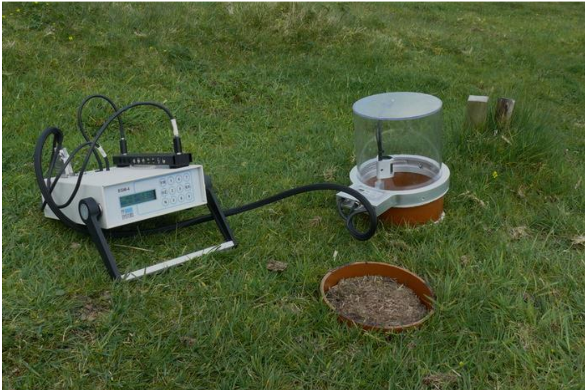
Picture 2.2. Portable IRGA connected to cylindrical Perspex chamber placed on top of a PVC collar recording soil CO 2 flux measurements
