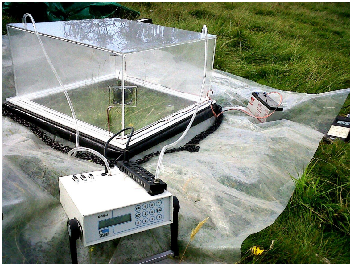
Picture 2.3. Net ecosystem CO 2 exchange measurements setup, including the Perspex chamber, battery, IRGA and the PAR Quantum device
