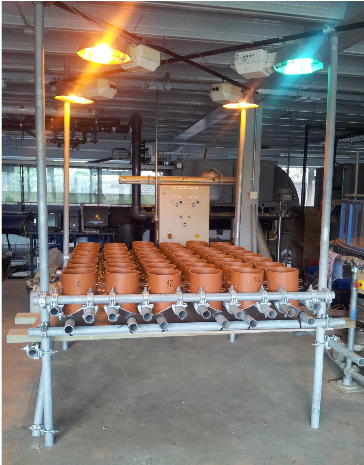
Picture C1-1. The completed frame, lighting system and all 48 pots, before the soil was added.
