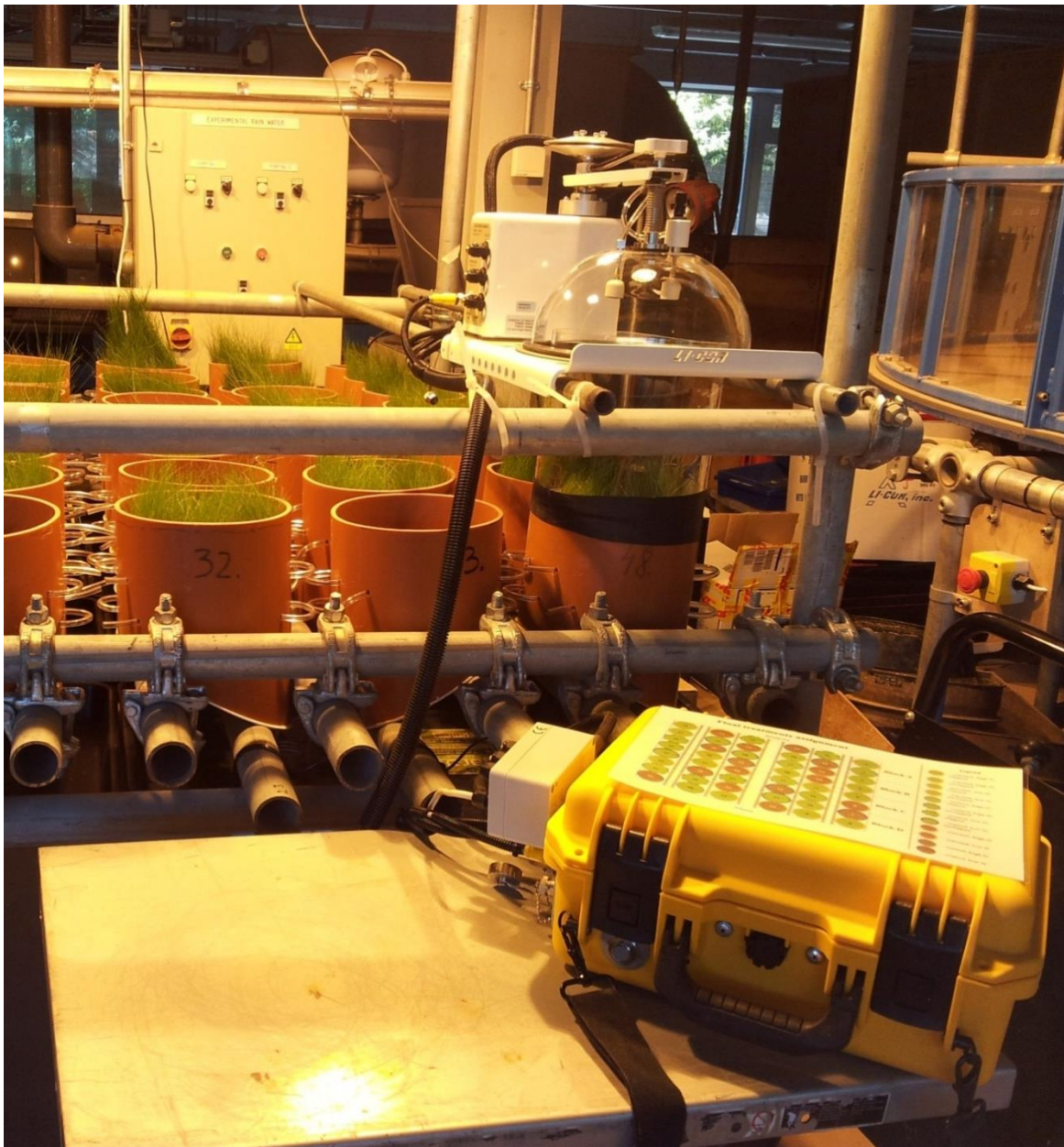
Picture 4.1. Illustration of the LI-Cor and lysimeter system used to record ecosystem CO 2 flux measurements.
