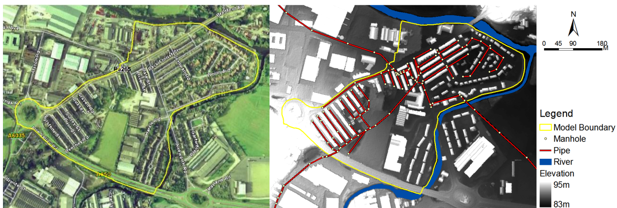
Figure 1. The satellite image (left, from Google Earth) and the DTM with buildings and sewer network (right) of Stockbridge area.
