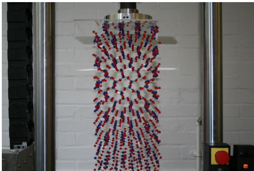
Figure 8.1 - A macro scale model of \alpha -cristobalite being tested under compression.
