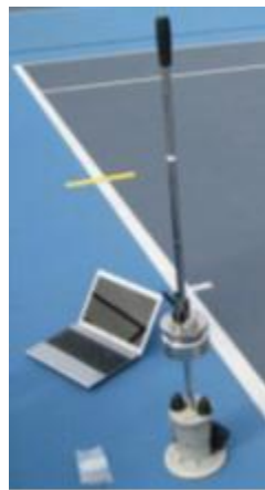
Figure 4.3: The Lightweight Deflectometer device
