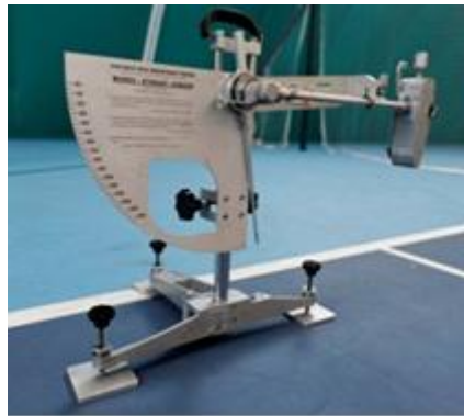
Figure 3.3: The pendulum test device
