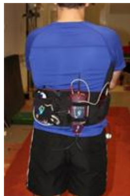
Figure 4.4: Placement of the belt, worn by participant, containing the data acquisition box, synchronisation box and battery
