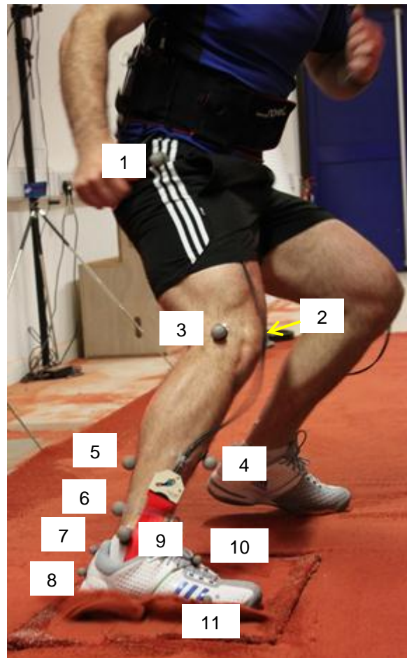
Figure 3.10: Joint coordinate system marker locations: 1) hip (greater trochanter) , 2) medial knee (medial femoral epicondyle), 3) lateral knee (lateral femoral epicondyle), 4) shin (anterior aspect of shank), 5) Achilles 1 (proximal bisection of posterior shank), 6) Achilles 2 (distal bisection of the posterior shank), 7) calcaneus 1 (proximal bisection of the calcaneus), 8) calcaneus 2 (distal bisection of the calcaneus), 9) lateral malleolus, 10) toe (base of 2 nd metatarsal), 11) 5 th metatarsal phalange
