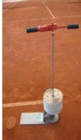
Figure 3.5: The rotational traction test device
