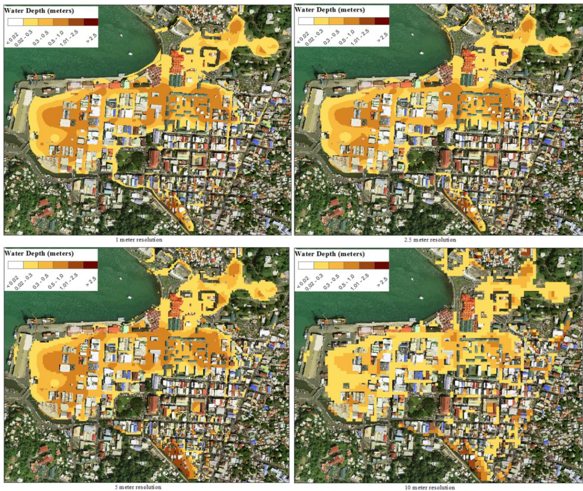
Figure 8-5: Max flood depths of the simulated event for model resolutions of 1.0, 2.5, 5.0 and 10.0 meters
