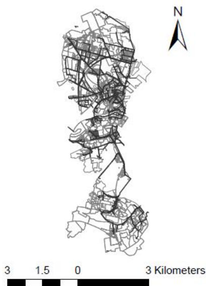
Figure 7-1: Setup of sewer model for Aarhus.
