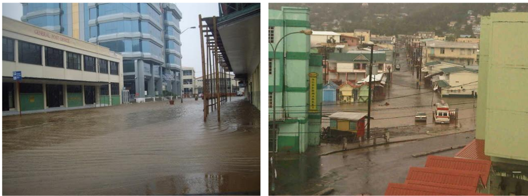
Figure 8-4: Example of the images used to extract water depths and extents for comparing to model results. In first image for example the depth is approximately 0.4m and the second image was used to extract extent since the water depth is not the same throughout the area
