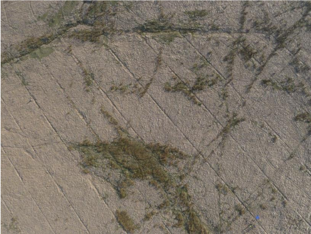
Figure 3.8: Visible aerial photography collected from a QuestUAV fixed wing aircraft flying at 100 m altitude over the Aclands catchment in March 2012. Linear features running from the top left of the image to the bottom right of the image show the anthropogenic drainage network.
