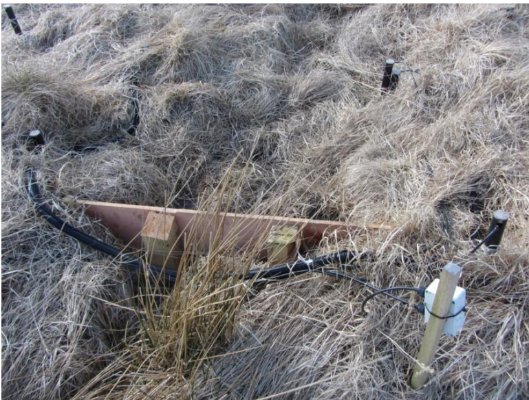
Figure 3.19: Close up of ditch block at S1 monitoring location in Spooners catchment, March 2013.
