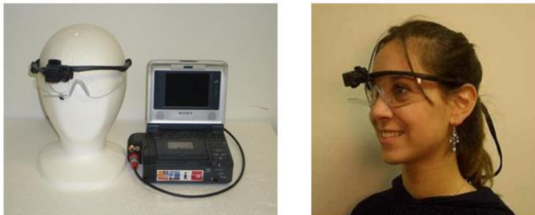
Figure 4 The Applied Science Laboratories Mobile Eye eye-tracker
