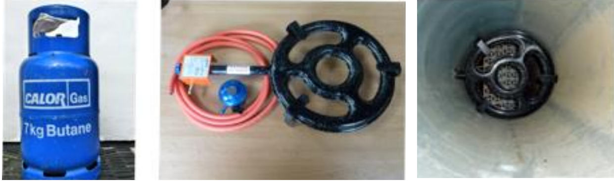
Figure 12 Left, the gas supply, center the Garcima paella gas burner used to simulate the igniters and right the burner fitted into the ventilation tube.
