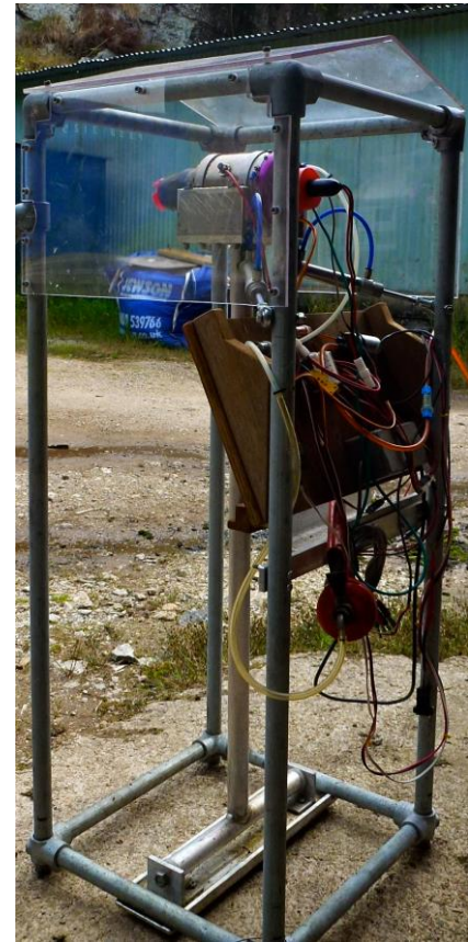
Figure 2 Operating system for the gas turbine, fuel pump, gas solenoid, fuel solenoid, Servo Control Board and Engine Control Unit.
