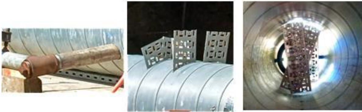
Figure 8 View of the hot exhaust gas inlet and the baffling act as diffusers to promote turbulent mixing
