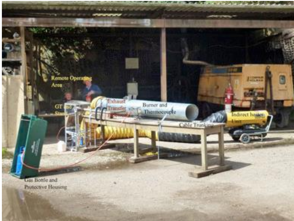
Figure 15 Final experimental setup for the VamTurBurner© prototype test, upper, set up of all equipment, lower, aerial view of risk assessment.
