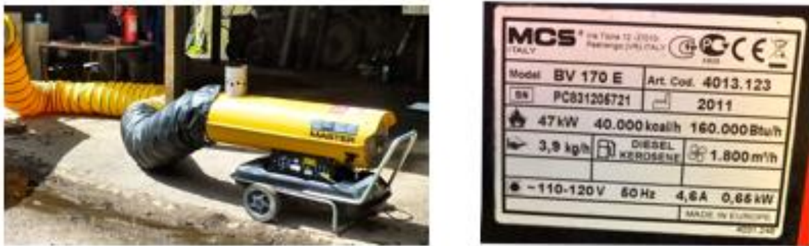
Figure 9 The preheating was simulated by an industrial heater (The Master BV 170 E Indirect Heater), which can be seen connected to the simulated mine ventilation tubing in Fig. 7.
