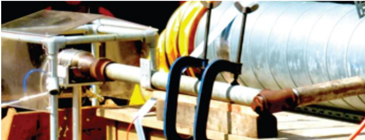
Figure 7 The exhaust gas was directed through the side of the vent chamber to allow for the input of the simulated ventilation air and preheating system to be attached from the end. The two gas flows merge prior to interaction with the igniters.
