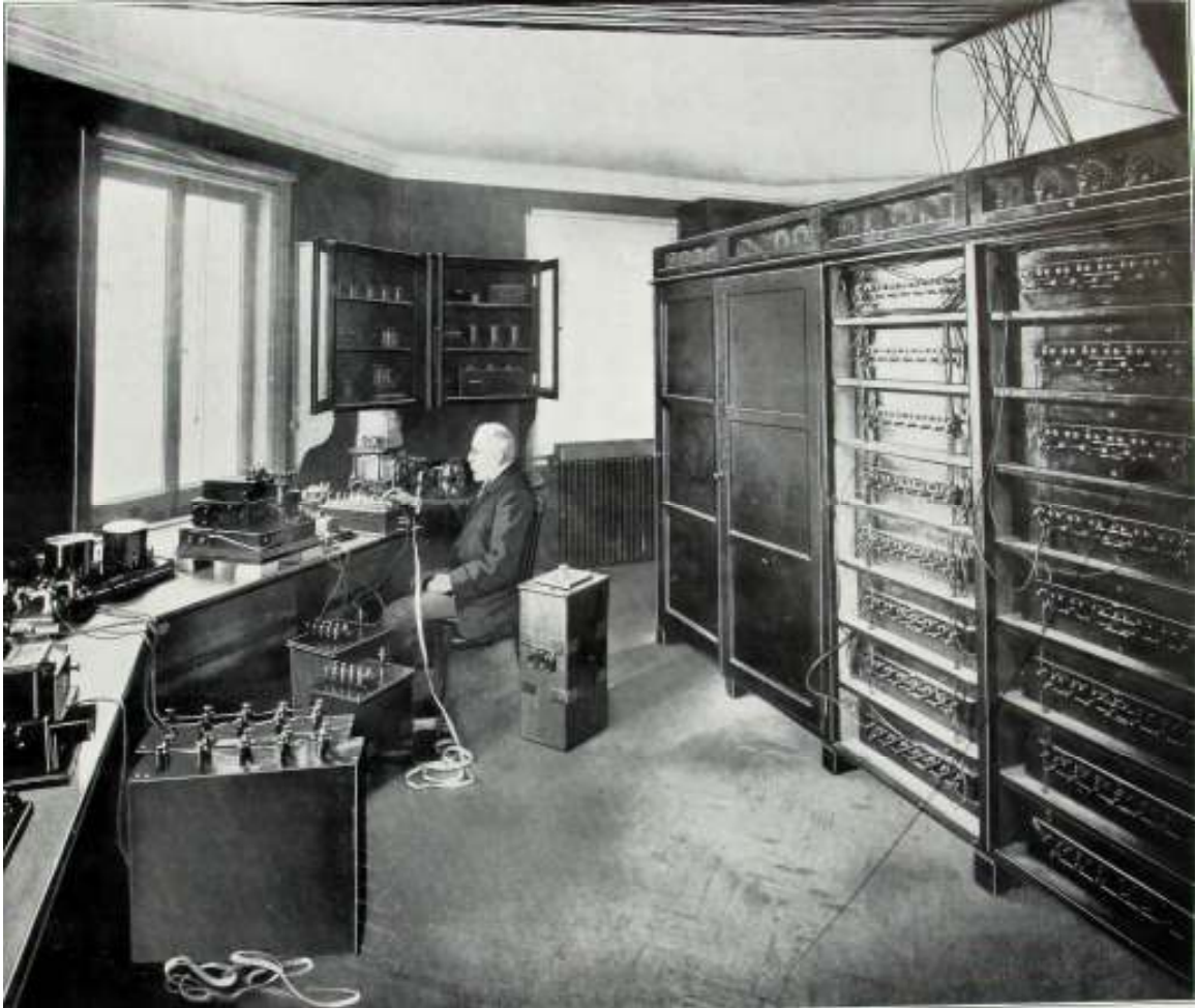
FIGURE 3: The Electra House laboratory in 1902. Here the Electrician-in-Chief Henry Saunders is seen testing the performance of a siphon recorder whose paper tape trails onto the floor. Behind him looms a large cabinet housing the ‘artificial line’: Anon., ‘Electra House: the New Home of the Eastern and Associated Telegraph Companies’, Builder’s Journal and Architectural Record , 20 August 1902, pp. 1-13, p. 10 (Image courtesy of Porthcurno Telegraph Museum).
