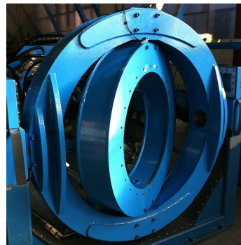
(a) Gimble system, tilted inner ring
