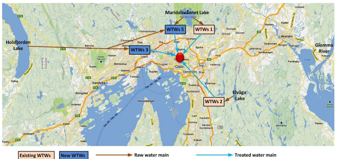
Figure 12: Layout of Oslo water supply system for intervention option C1
