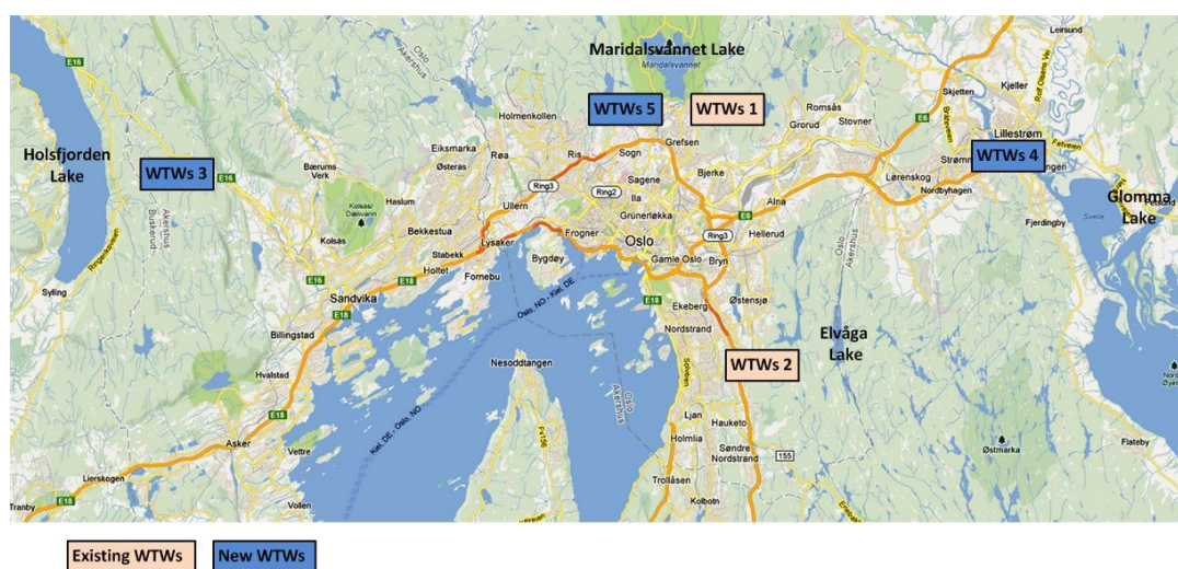
Figure 4: General layout of the existing and new WTWs and water resources in Oslo case study
