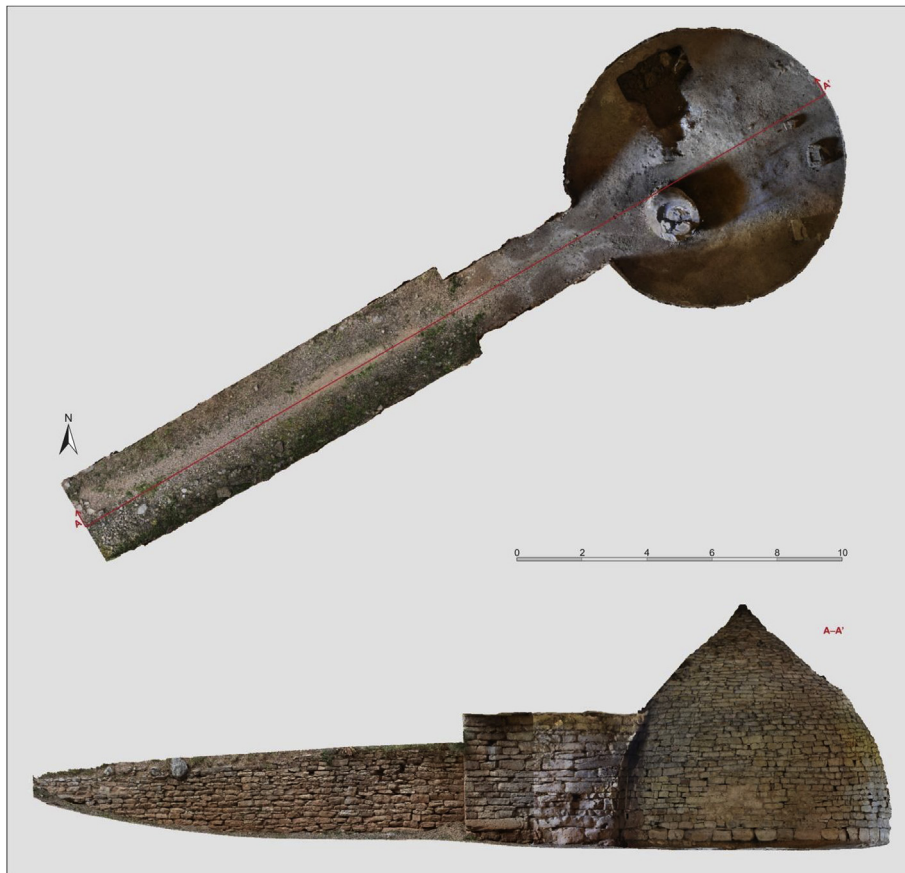
Fig. 9. Tiryns, tholos tomb. Plan and section derived from the 3D photogrammetry model. (J. Pakkanen – A. Brysbaert).
