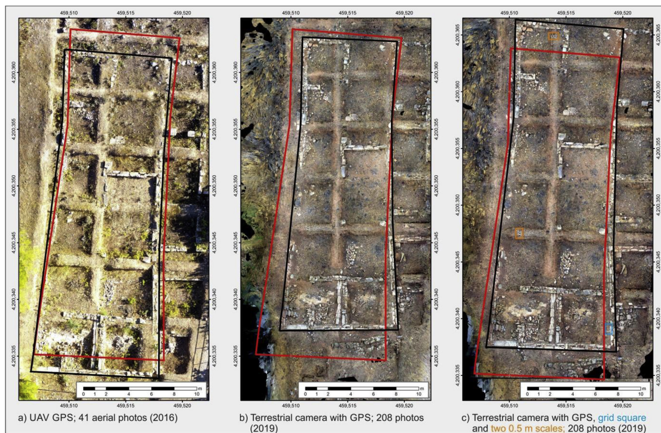
Fig. 3. Salamis, Oikia Theta. Comparison of photogrammetry results georeferenced using inbuilt GPS receivers. Red: outline of the house remains georeferenced with a DGPS. Black: house outline based on the tested set of photographs. (J. Pakkanen). (For interpretation of the references to colour in this figure legend, the reader is referred to the Web version of this article.)
