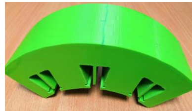
Fig. 9. Back-iron extension dummy stator for winding trials
