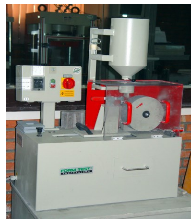
Fig 3 Abrasion test apparatus based on EN standard
