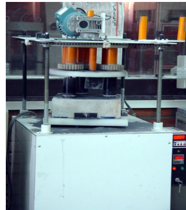
Fig 2 Manufactured revolving disk apparatus based on ASTM standard
