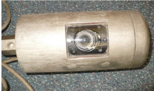
Figure 18. Endoscopic camera head with infrared diodes
