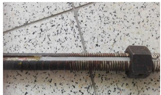
Figure 17. Instrumented bolt – the groove fragment with tensometers attached
