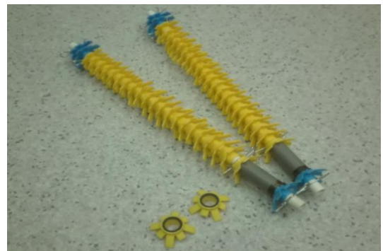
Figure 16. Measuring anchors of extensometric probe
