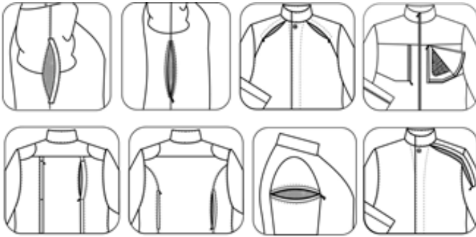
Fig. 20. Examples of varieties of slot-like ventilation elements in protective clothing
